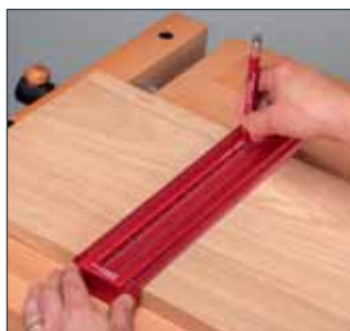
Parallelrisse in 1 mm Abstand
