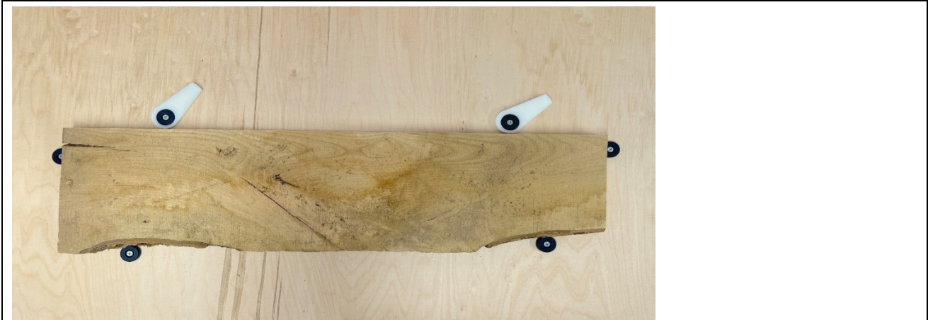
Figure 89: Fixing a wooden board to the work plate (as an example)
