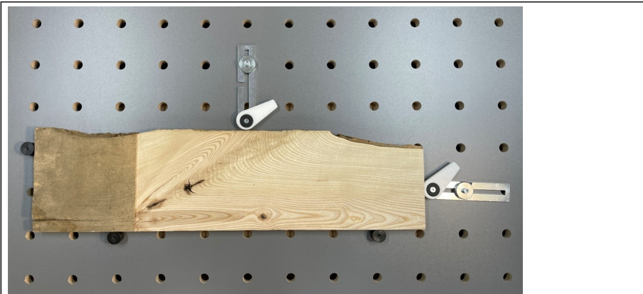
Figure 90: Fastening a wooden board to the hole matrix board
