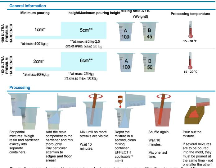
Observe the maximum layer heights when pouring and only ever mix the required quantities. Do not use any other additives, such as deaerators (these can have a negative effect on the properties of the resin - for example, they can cause clouding. Thick layers and high temperatures cause the material to harden faster than specified. The mixture also becomes hotter, which can result in yellowing, boiling bubbles, stress cracks and increased shrinkage.
