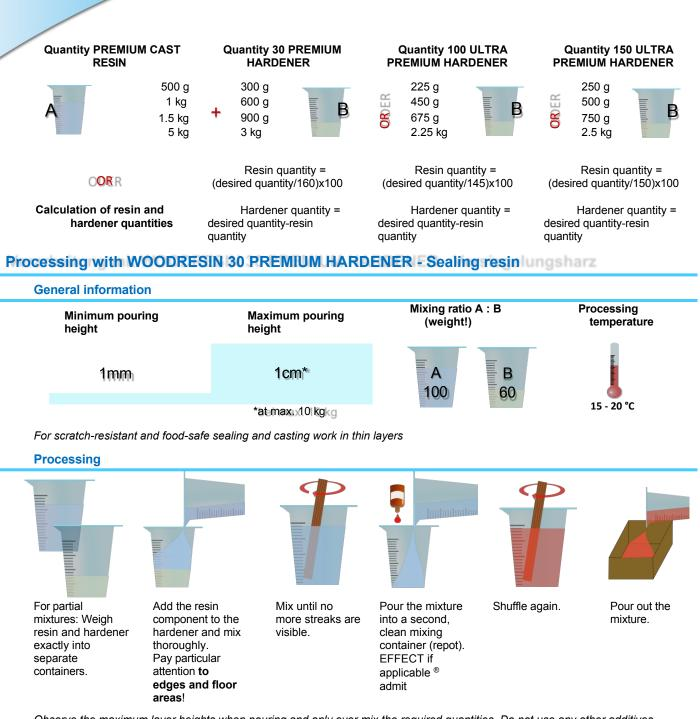
Observe the maximum layer heights when pouring and only ever mix the required quantities. Do not use any other additives, such as deaerators (these can have a negative effect on the properties of the resin - for example, they can cause clouding. Thick layers and high temperatures cause the material to harden faster than specified. The mixture also becomes hotter, which can result in yellowing, boiling bubbles, stress cracks and increased shrinkage.
